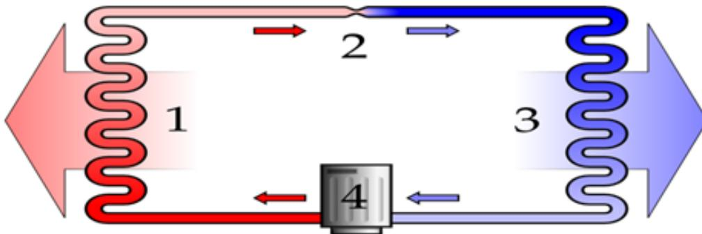
Fig. 1 Diagram of a phase change heat pump: 1) condenser coil 2) expansion valve 3) evaporator coil and 4) compressor.
