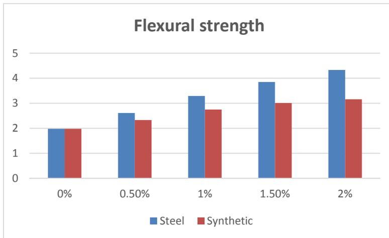
Fig. 3. Flexural strength of 28-days concrete
