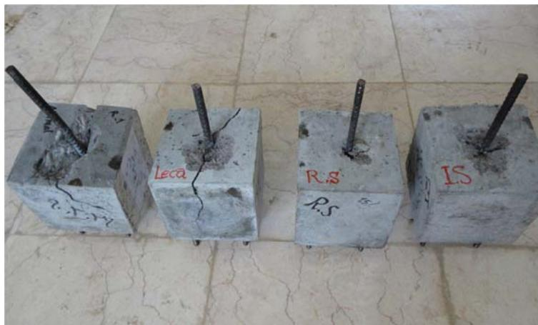
Fig. 5. Pullout test.
