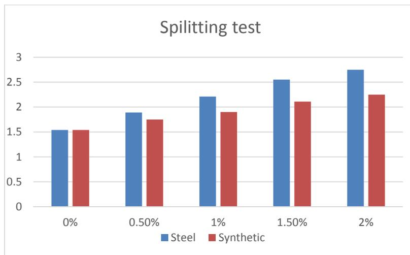
**Fig. 2. Splitting tensile strength of 28-days concrete**
