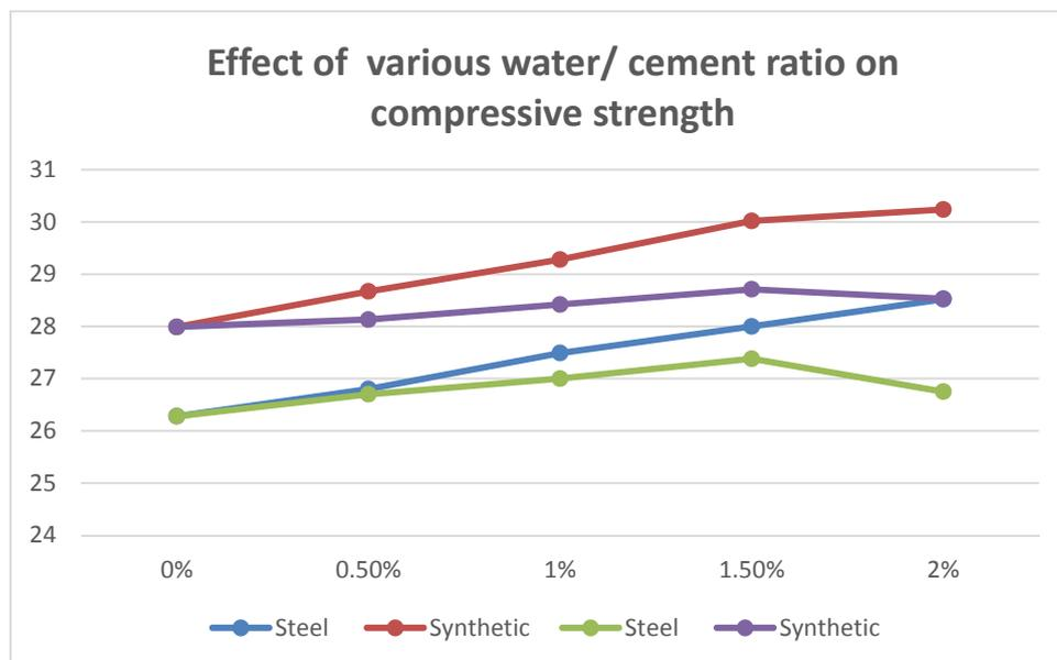
Fig. 4. Effect of various water/ cement ratio on compressive strength with various fiber
