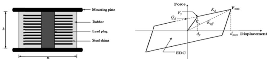
Fig. 2 LRB system and bilinear model of LRB
