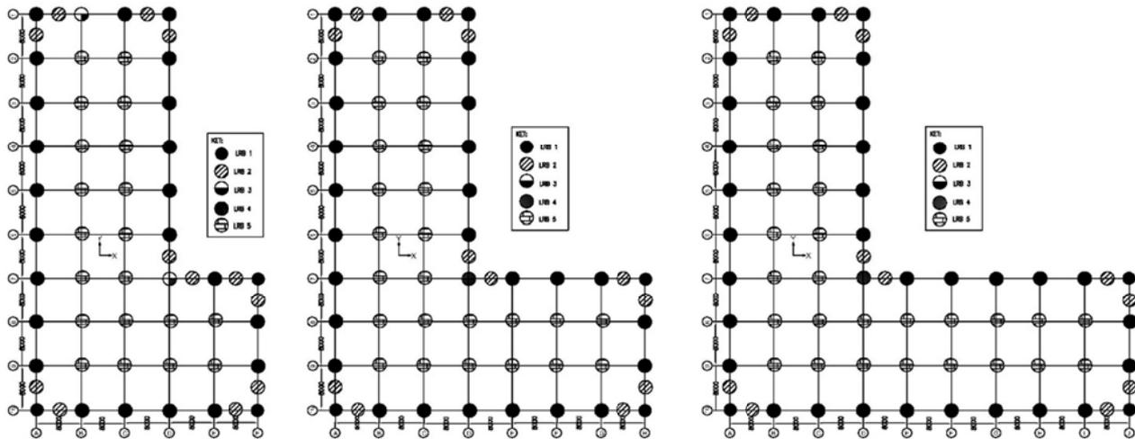
Fig. 4 Layout of base isolation on L1, L2, and L3 models
