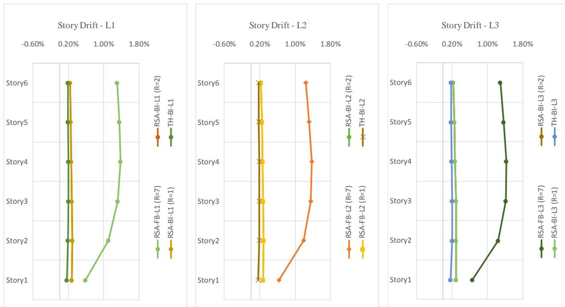
**Fig. 7** The comparison drift story of fixed base and base-isolated on each models
