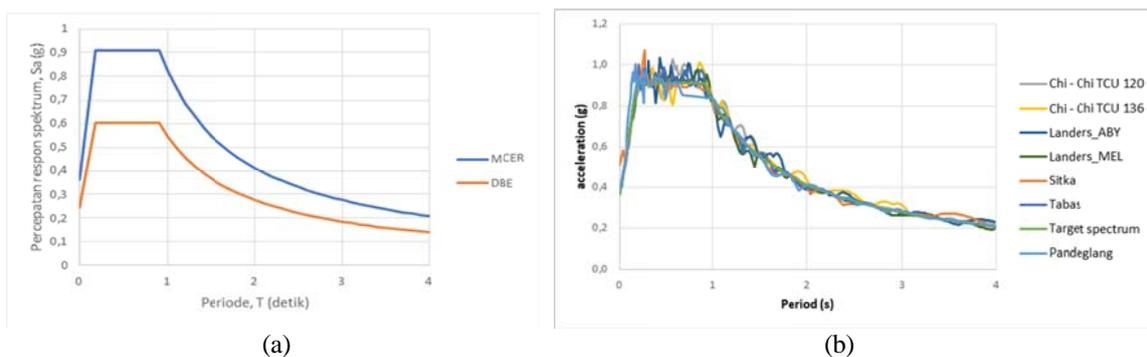
Fig. 5 The comparison of DBE and MCER spectrum (a); seven selected ground motion are matching to target spectrum MCER (b)
