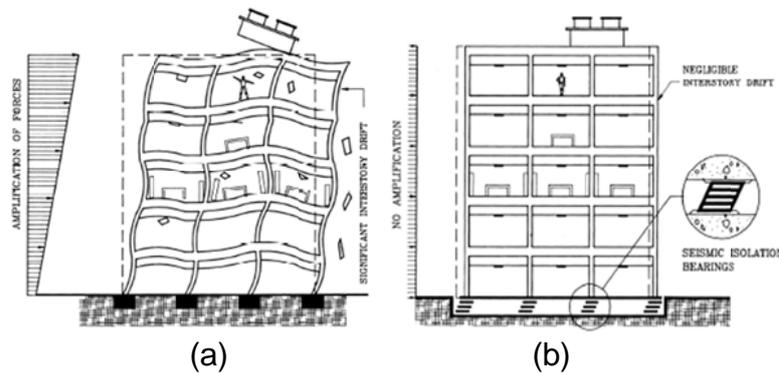
Fig. 1 Conventional structure / fixed base (a), Base-isolated structure (b)
