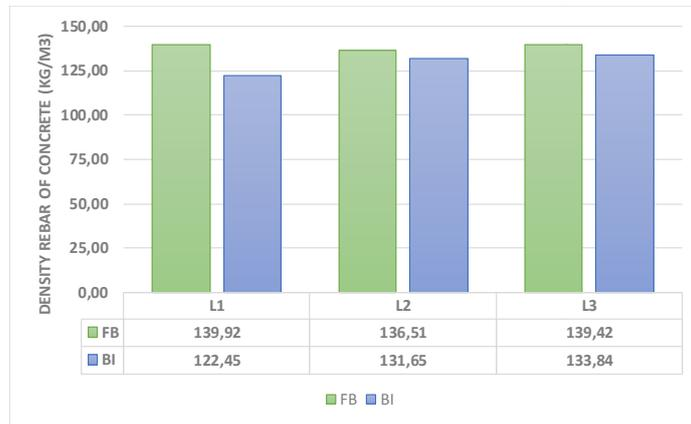
**Fig. 8** The comparison of density rebar of a cubic concrete ( $\text{kg/m}^3$ ) of fixed base and isolated base
