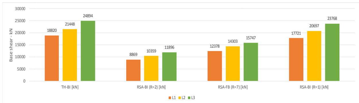
**Fig. 6** The comparison base shear of fixed base and base-isolated
