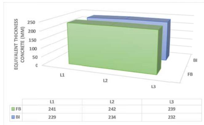
**Fig. 9** The comparison of equivalent thickness concrete of fixed base and isolated base
