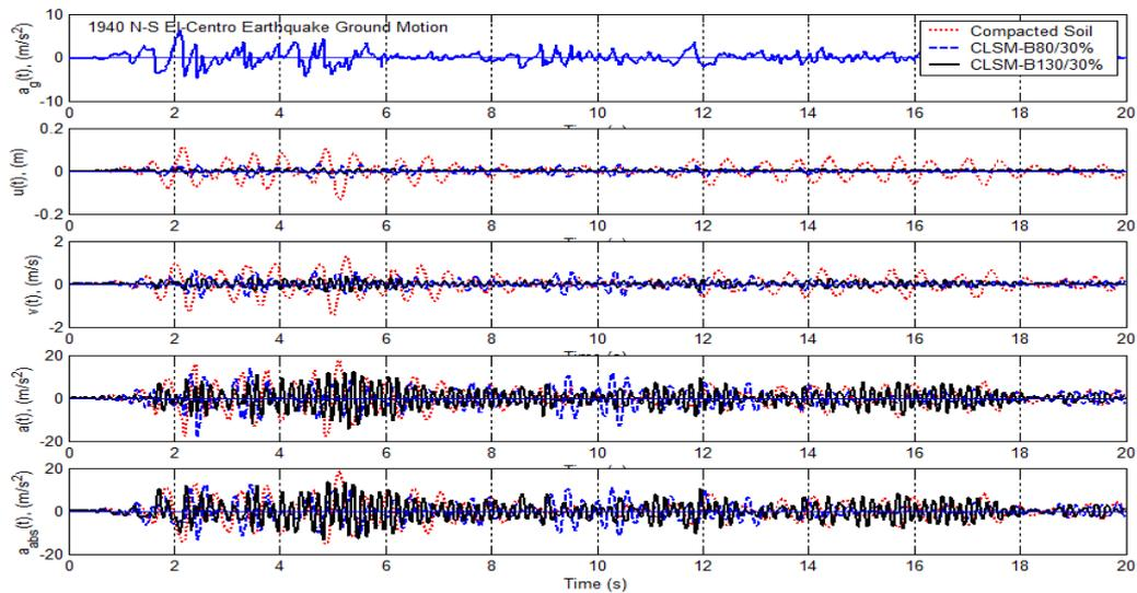
Fig. 6 Calculated vertical responses of node 181 of trench duct backfilled with three different backfill materials with damping subjected to 1940 EI-Centro NS ground acceleration.
