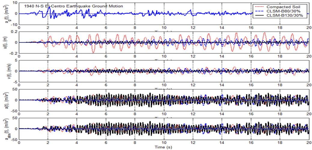
Fig. 5 Calculated vertical responses of node 181 of trench duct backfilled with three different backfill materials without damping subjected to 1940 EI-Centro NS ground acceleration.
