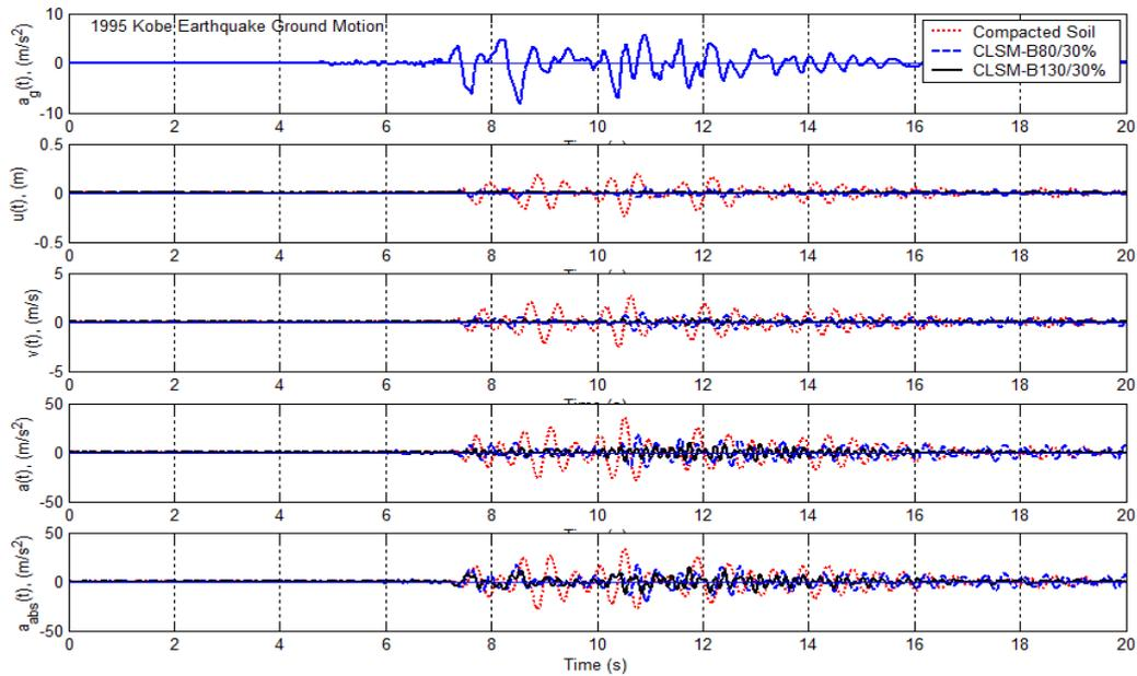
Fig. 8 Calculated vertical responses of node 181 of trench duct backfilled with three different backfill materials with damping subjected to 1995 Kobe ground acceleration.
