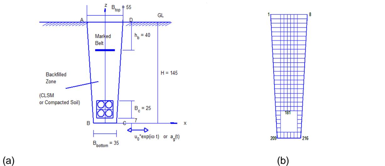
Fig. 1 (a) Schematic of a trench duct with backfill (length unit:cm); (b) finite element mesh of a trench duct (171 quadrilateral elements with 216 nodes)
