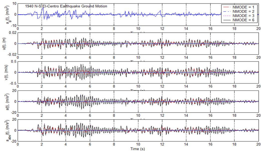
Fig. 4 Calculated vertical responses of node 181 of trench duct backfilled with CLSM-B130/30% with damping subjected to 1940 EI-Centro NS ground acceleration.
