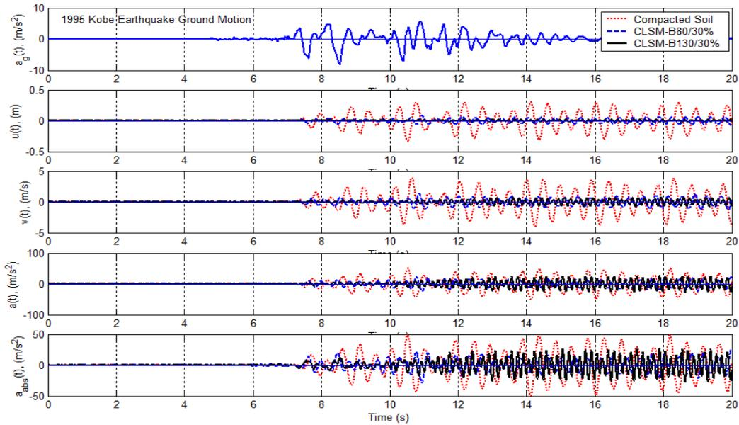
Fig. 7 Calculated vertical responses of node 181 of trench duct backfilled with three different backfill materials without damping subjected to 1995 Kobe ground acceleration.
