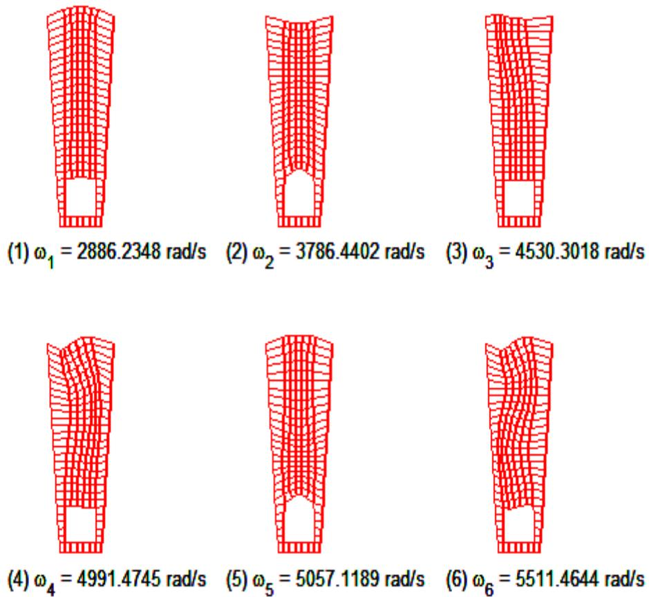
Fig. 2 Natural modes of trench ducts backfilled with CLSM-B130/30%
