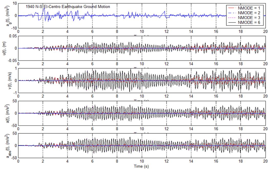
Fig. 3 Calculated vertical responses of node 181 of trench duct backfilled with CLSM-B130/30% without damping subjected to 1940 EI-Centro NS ground acceleration.
