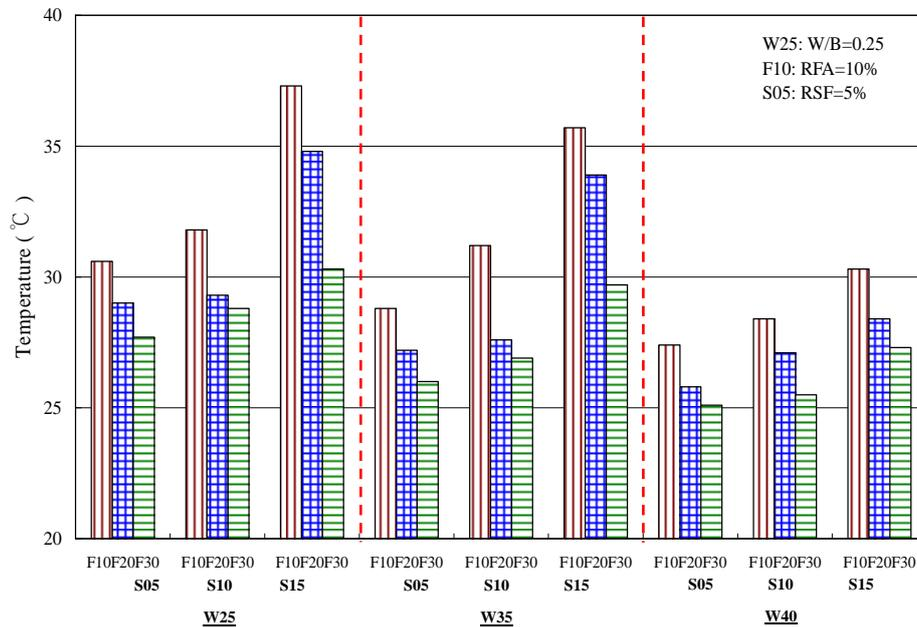
Fig. 9 Relations between maximum central temperature of specimens and the W/B ratio
