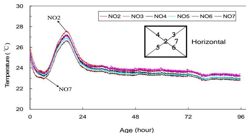
Fig. 5 Temperature distribution in horizontal direction for specimen W35-S10-F20
