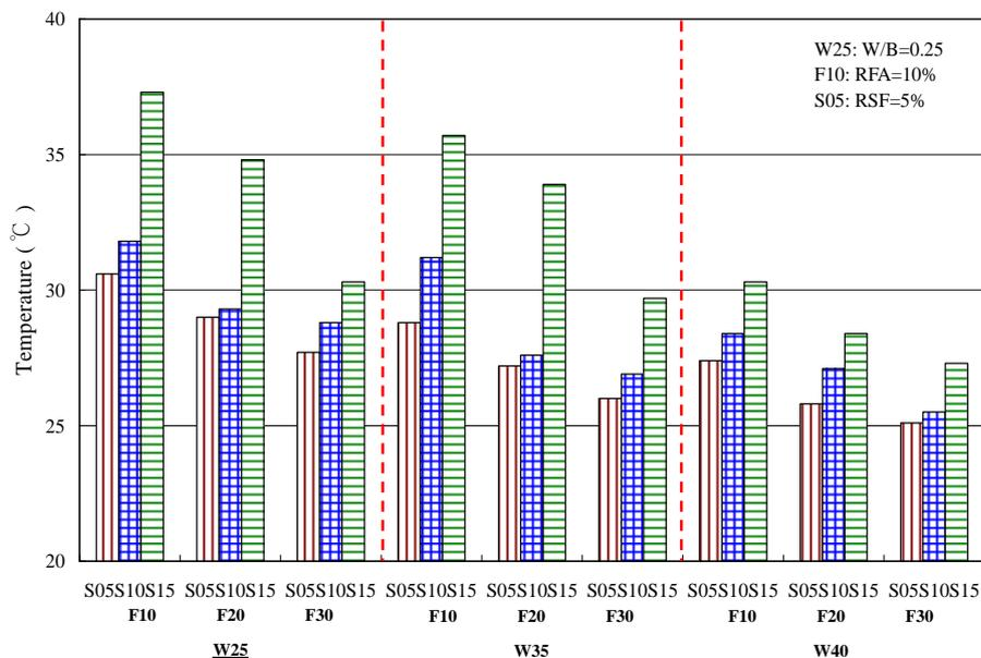
Fig. 8 Relations between maximum central temperature of specimens and the RSF ratio
