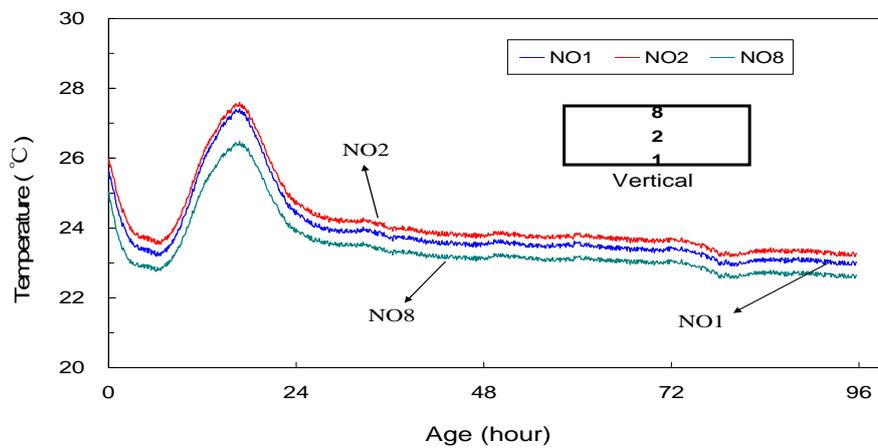
Fig. 4 Temperature distribution in vertical direction for specimen W35-S10-F20
