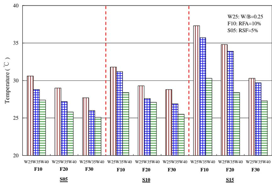
Fig. 7 Relations between maximum central temperature of specimens and the W/B ratio
