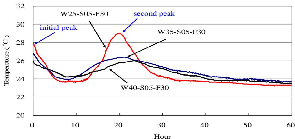
**Fig. 6** Temperature development at the center of specimen with different W/B
