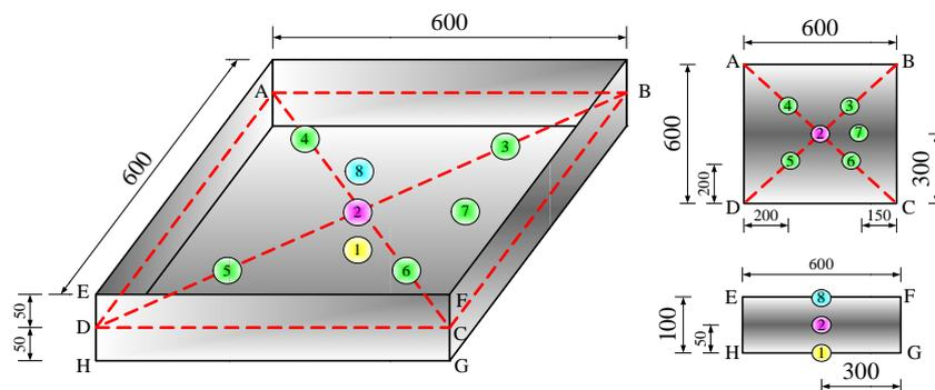
Fig. 2 Location of embedded thermistors in specimen
