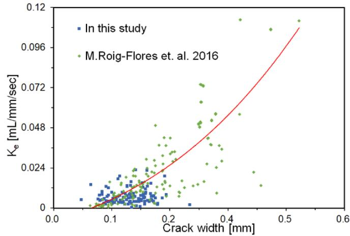
Fig. 2 Initial Crack width- $K_e$  result
