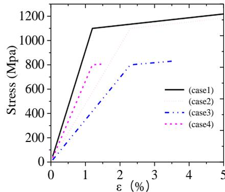
Fig. 11 Load-strain curves of the hanger
