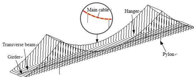
**Fig. 9** FE model of the bridge
