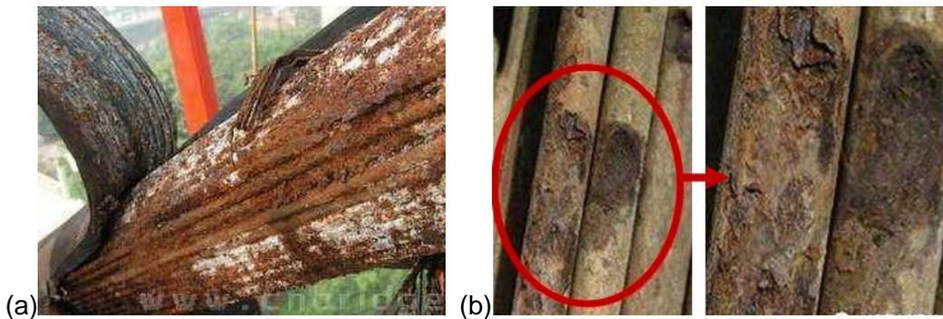
Fig. 2 Corrosive types of steel wire: (a) uniform corrosion (b) pitting corrosion
