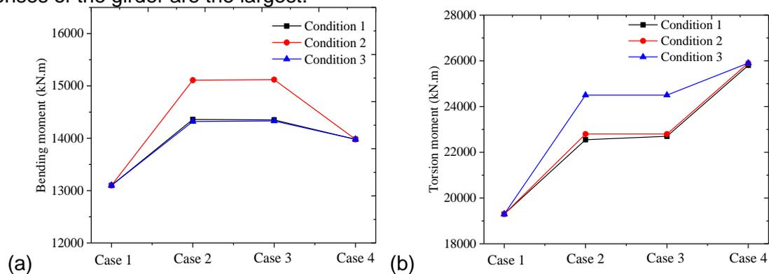
Fig. 15 Maximum responses of the girder (a) near the broken hanger (b) near the tower
