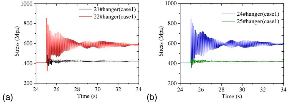
**Fig. 12** hangers responses to the breakage of one hanger
