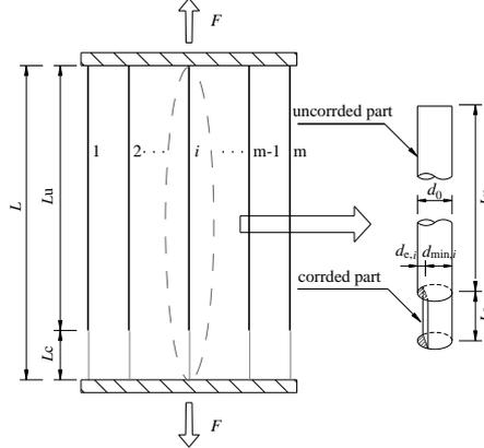
Fig. 5 Modified model of a hanger
