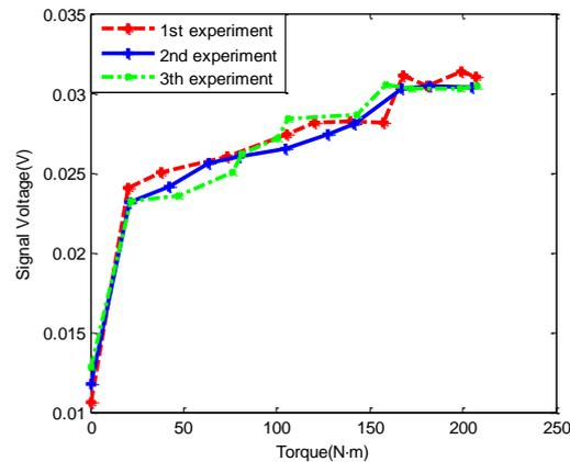
Fig. 10 Peak values of the eleven bolt pre-load conditions
