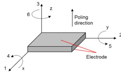
Fig. 2 The poling of PZT sensor in 3-direction
