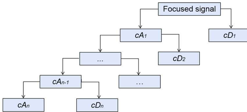
Fig. 5 The scheme of n-level wavelet decomposition
