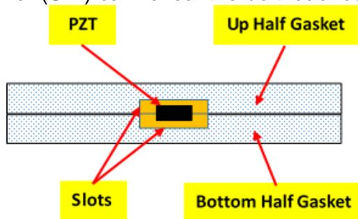
Fig. 3 The design of smart washer
