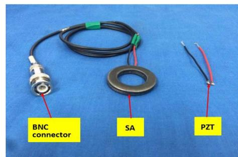
Fig. 4 Fabricated smart washer with a connecting BNC cable
