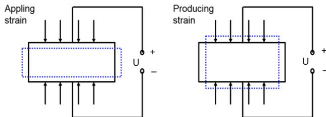
Fig. 1 Direct piezoelectric effect and converse piezoelectric effect
