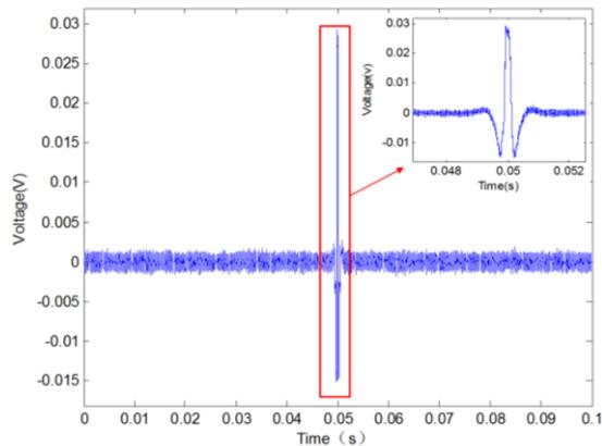
Fig. 9 The received signals with 167.5N·m applied torque
