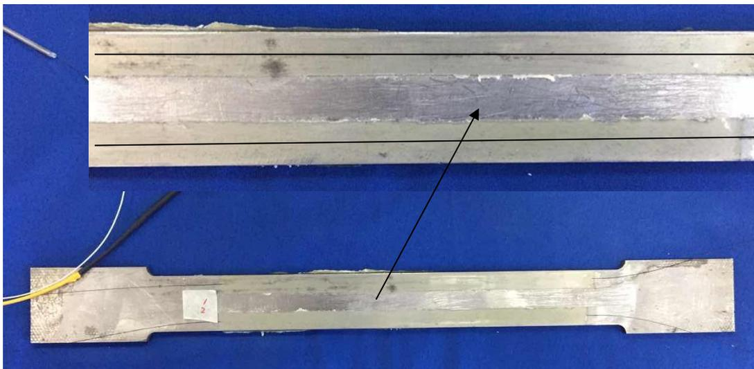
Fig.7 Steel plate used for the test of different shear modulus of adhesive
