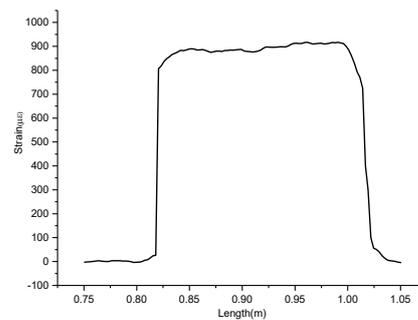
(b) Strain distribution with 1.5mm adhesive layer thickness
