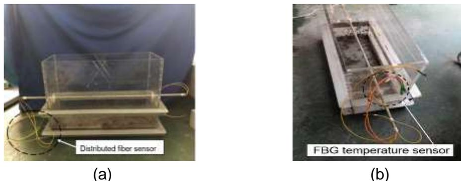
Fig. 2 Test pipeline installed sensors put into test box: (a) distributed fiber sensor; (b) FBG temperature sensor
