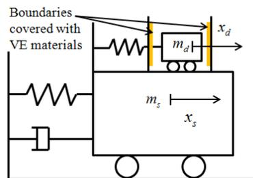
Fig. 1 Schematic of PTMD
