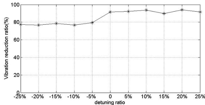
Fig. 6 Reduction ratio of differently tuned PTMDs
