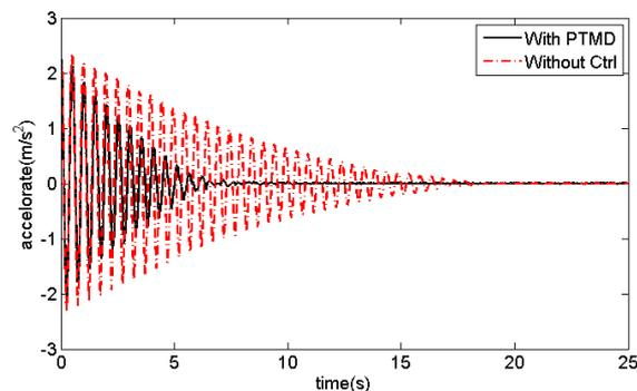
Fig. 4 Response of the primary structure controlled by PTMD in free vibration case
