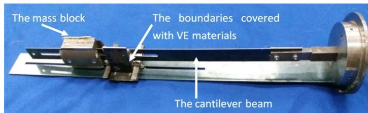
Fig. 3 The PTMD inside the steel rod.
