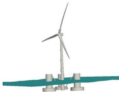
Fig. 3 NREL DeepCwind Semi-submersible type (Kang 2017)
