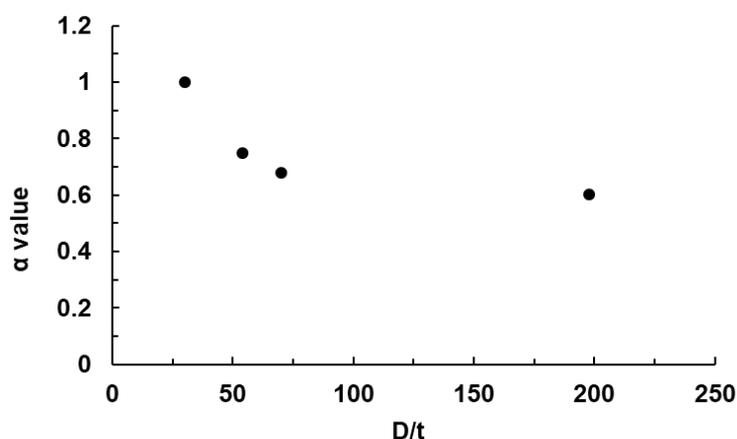
Fig. 1 Estimation of CFT creep function value based on previous study
