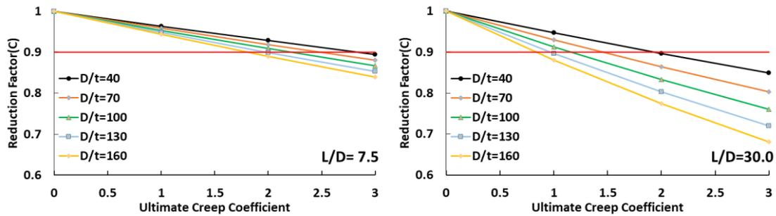
Fig. 3 Reduction of ultimate strength by creep at different slenderness ratio and D/t
