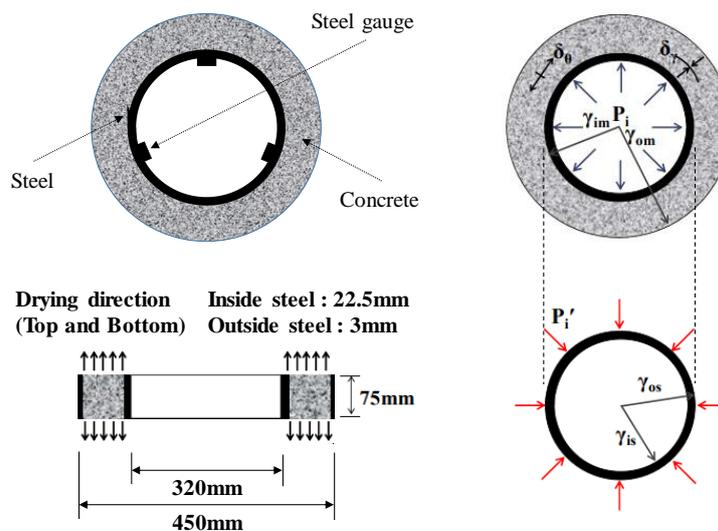
**Figure 2.** Overview of ring test (Restrained shrinkage strain)
