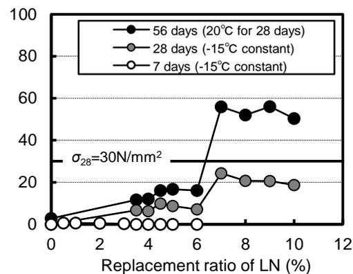
**Fig.7** Compressive strength (-15° C)
