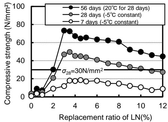
**Fig.5** Compressive strength (-5° C)
