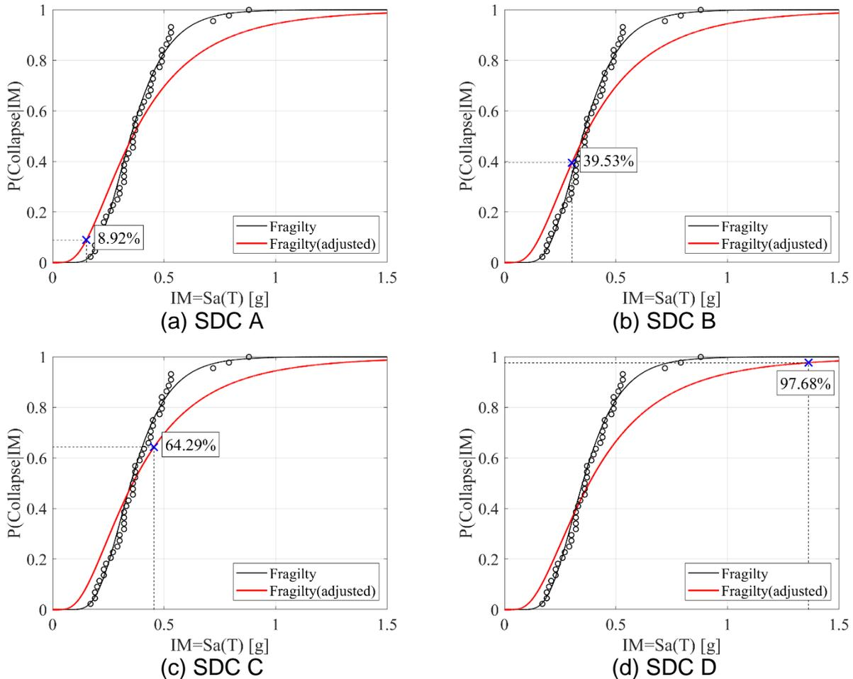
Fig. 5 Adjusted collapse fragility curve according to SDC
