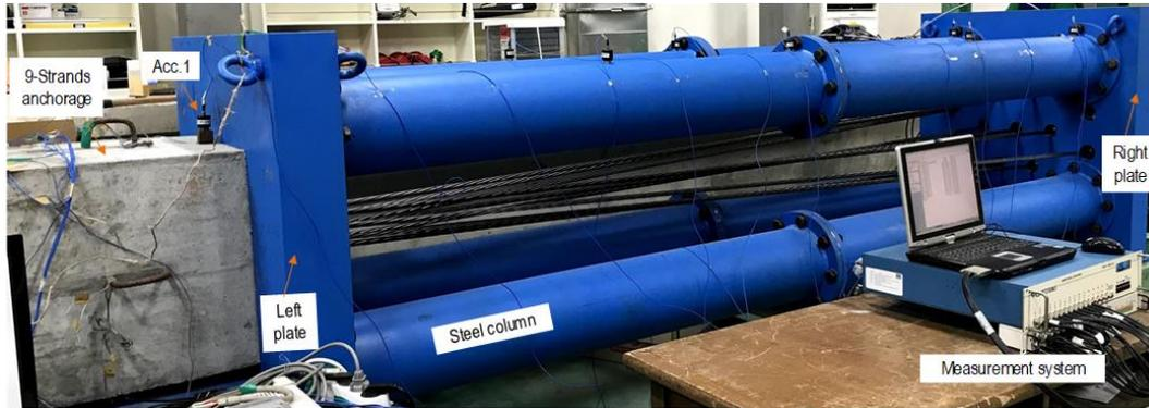
a) A lab-scale PSC structure and installation of accelerometers
