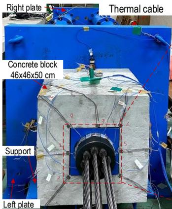
b) Test setup of concrete anchorage
