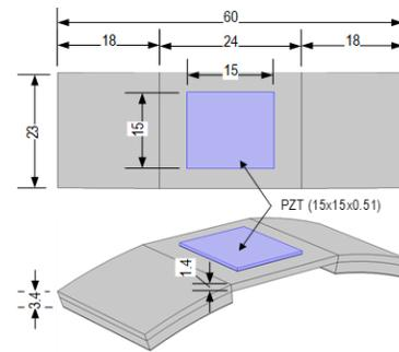
d) Geometric parameters of hoop-type PZT interface
