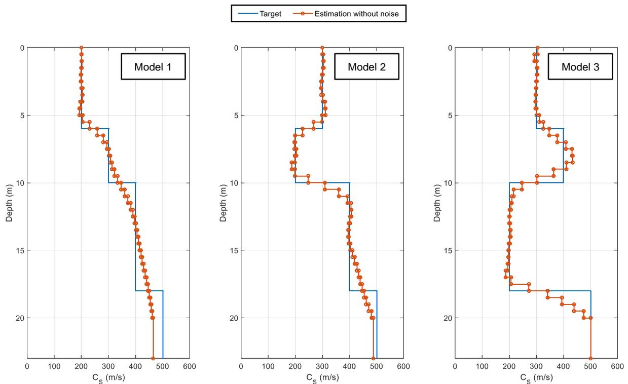
Fig. 1 Estimated profiles of shear-wave velocities in layered half-spaces
