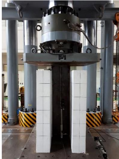
**Fig. 2** Push-out test set up with UTM
