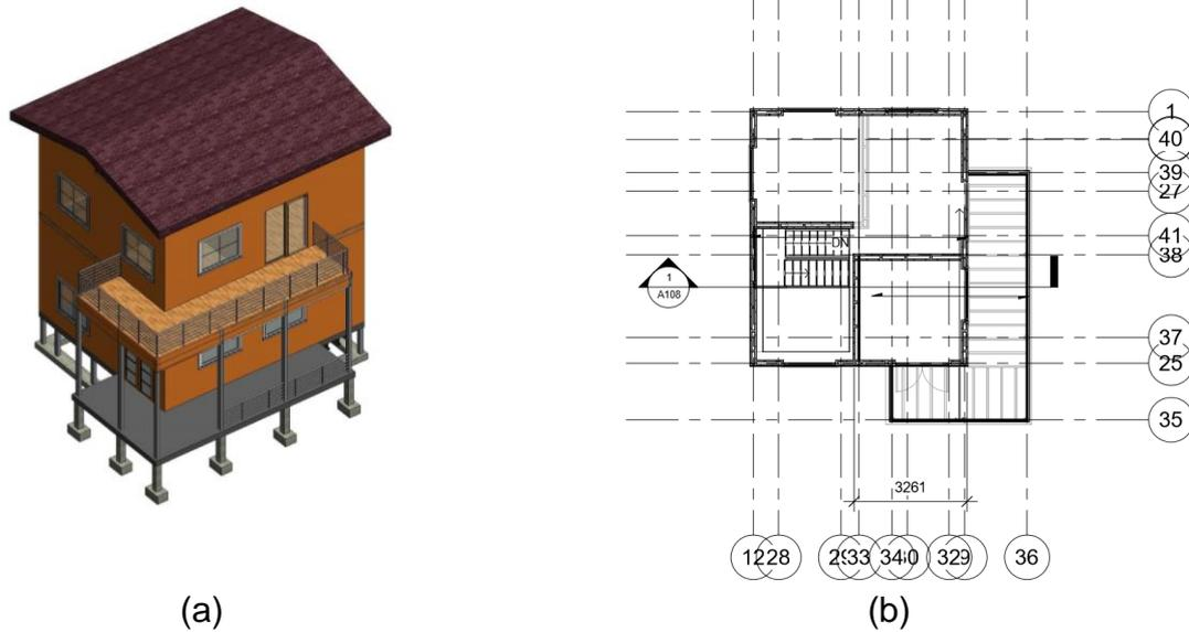
**Figure 3** Revit Model of low-rise CLBT buildings: (a) perspective view; (b) plan.
