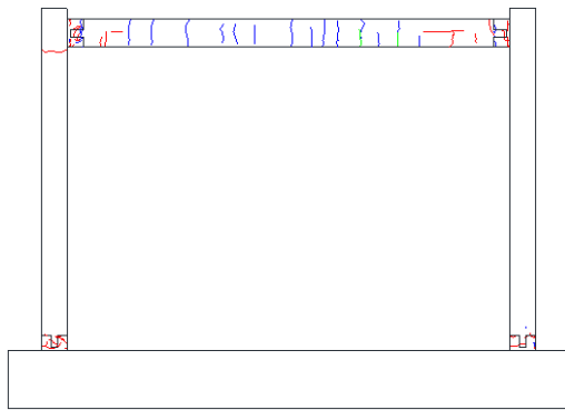
(a) Cracking aspect
