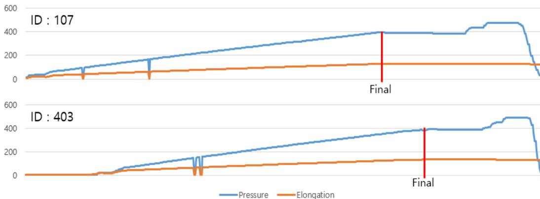
Fig. 3 Pressure and elongation data in real-time
