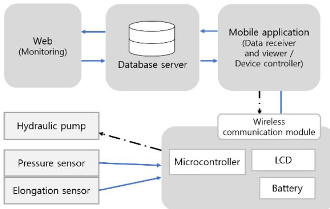
Fig. 1 System plan
