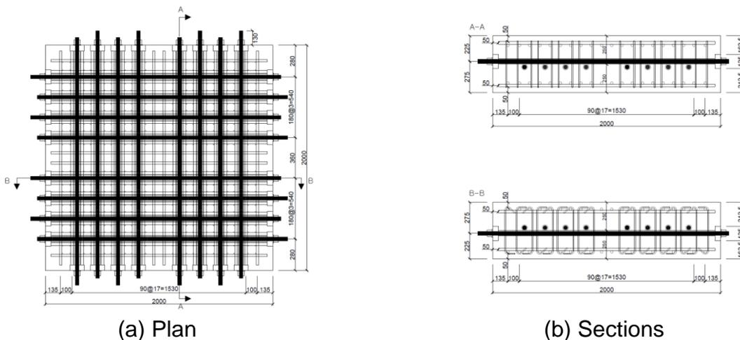
**Fig. 2** Details of unbonded post-tensioned concrete panel
