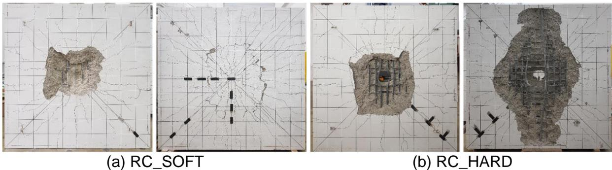
Fig. 4 Fracture mode of RC specimens
