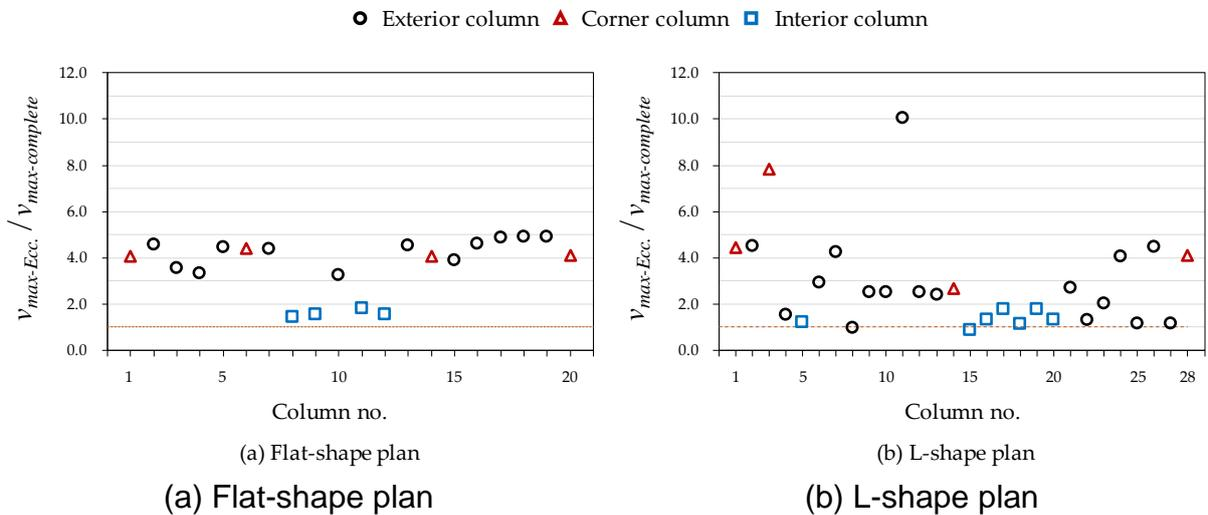
**Fig. 3** Maximum punching shear ratio according to the modeling method (gravity load only)
