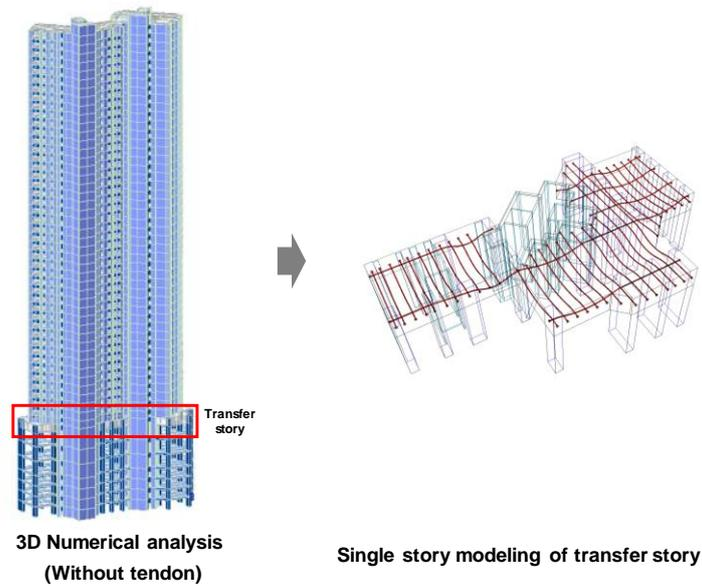
Fig. 1 Analysis and design process for post-tensioned transfer plate system
