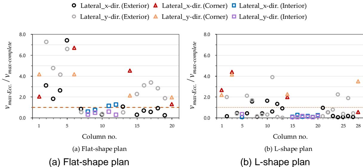
**Fig. 4** Maximum punching shear ratio according to the modeling method (lateral load only)
