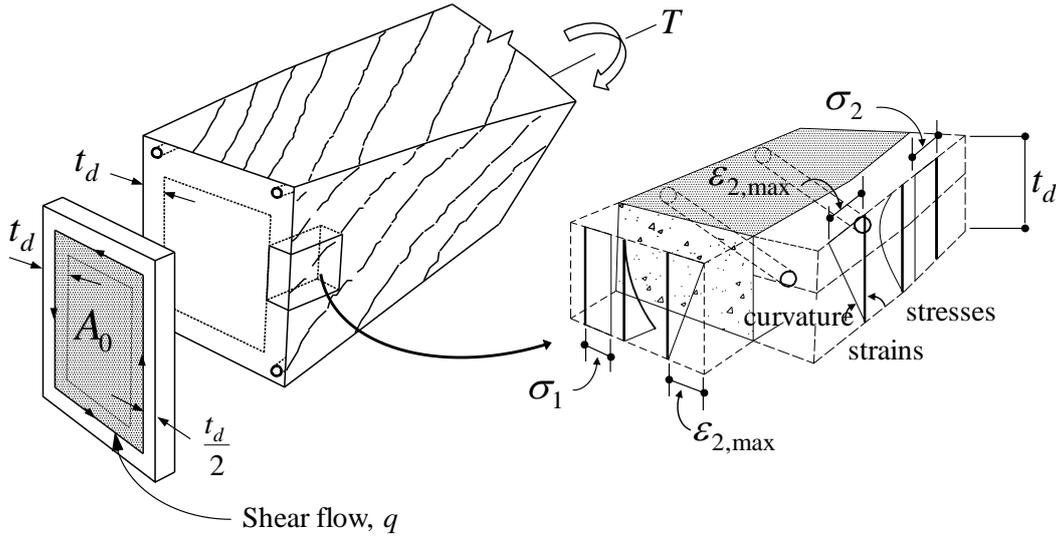
**Fig. 2** Torsional member and shear element within the effective thickness
