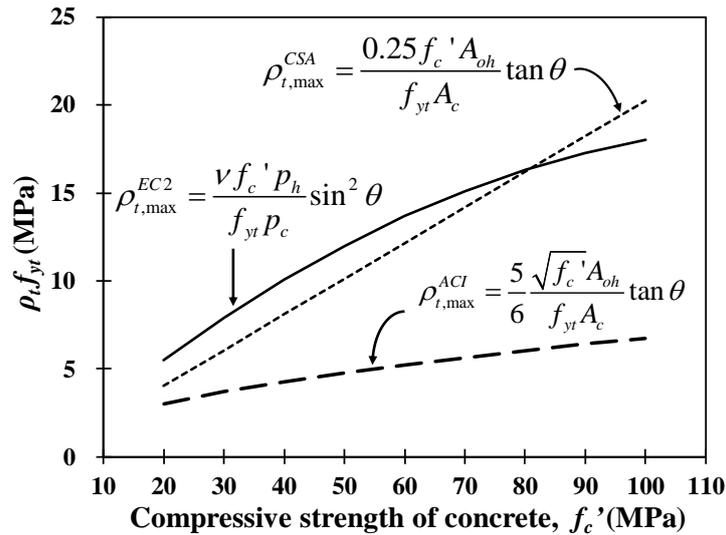
Fig. 1 Maximum torsional reinforcement ratios in design codes
