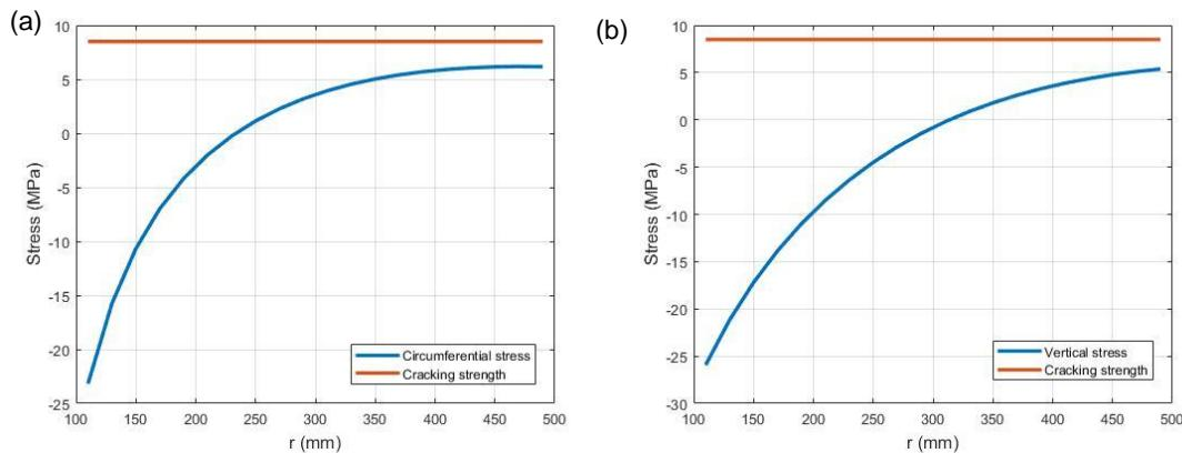
Fig. 4. Stress distribution along radial direction at the middle of the pile: (a) circumferential and (b) vertical stress.
