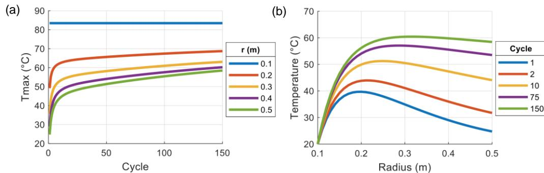
Fig. 2. (a) Maximum temperature of each loading cycle inside the pile;
