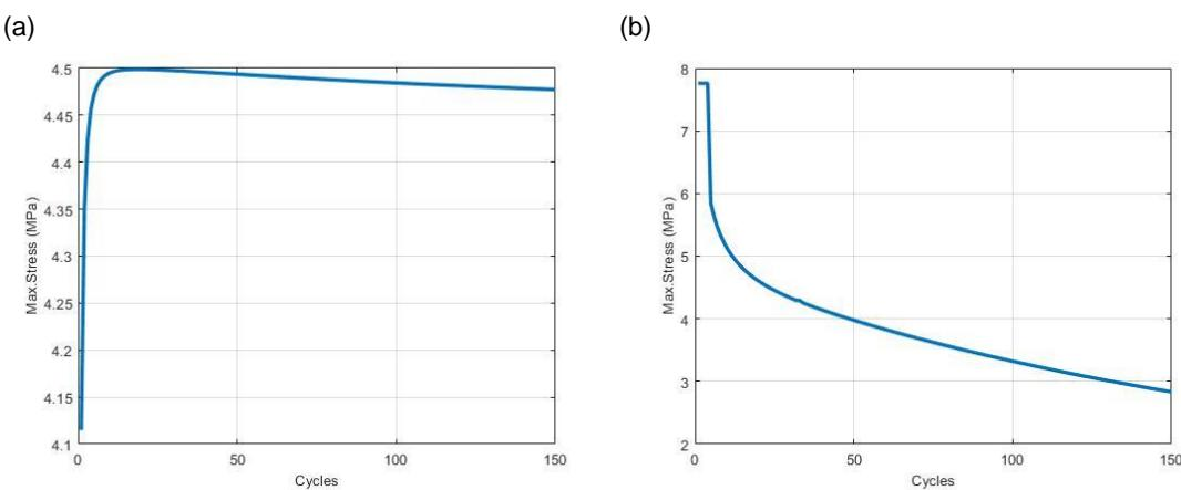
Fig. 3. Maximum circumferential stress distribution with cycles at the bottom of the pile at (a)  $r = 0.110\text{ m}$  and (b)  $r = 0.490\text{ m}$ .
