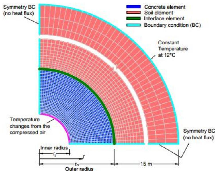
Fig. 1. The 2D plane strain model.
