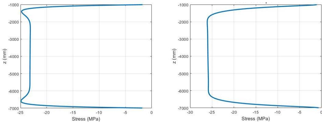
Fig. 5. Stress distribution along longitudinal direction at the inner skin of the pile: (a) circumferential and (b) vertical stress.
