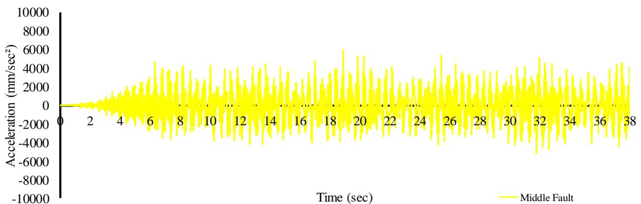
Fig. 12 Seismic accelerations on Point 11348 during middle fault earthquake for structure with NSC (according to EUROCODE standard).
