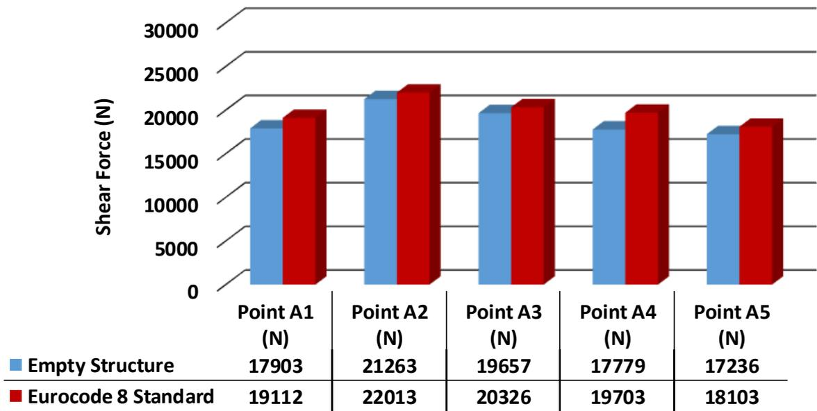
Fig. 9 Shear Forces along Axis A-A for middle-fault earthquake.
