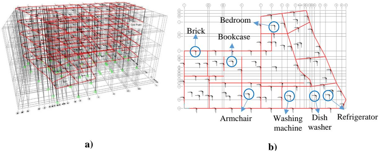
Fig. 5 Nonstructural component loads in the structure a) general view of nonstructural components b) nonstructural component loads of fifth floor .
