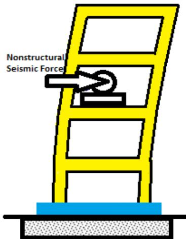
Fig. 1 Non-structural component force in the structure.
