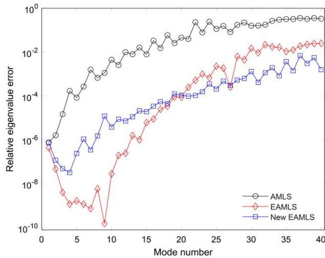
Fig. 3. Relative eigenvalue errors for the cantilever plate.
