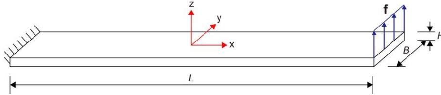
**Fig. 2.** Cantilever plate subjected to a shear load.
