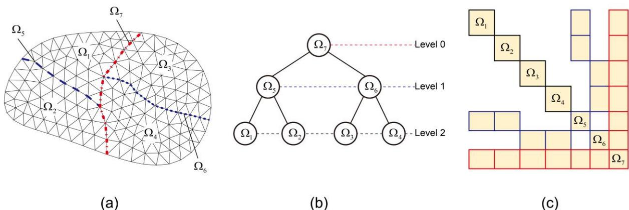
**Fig. 1.** Multilevel substructuring of a generic structure: (a) partitioned structure, (b) substructure tree, and (c) block matrix pattern for the reordered matrix (Hyun 2020).
