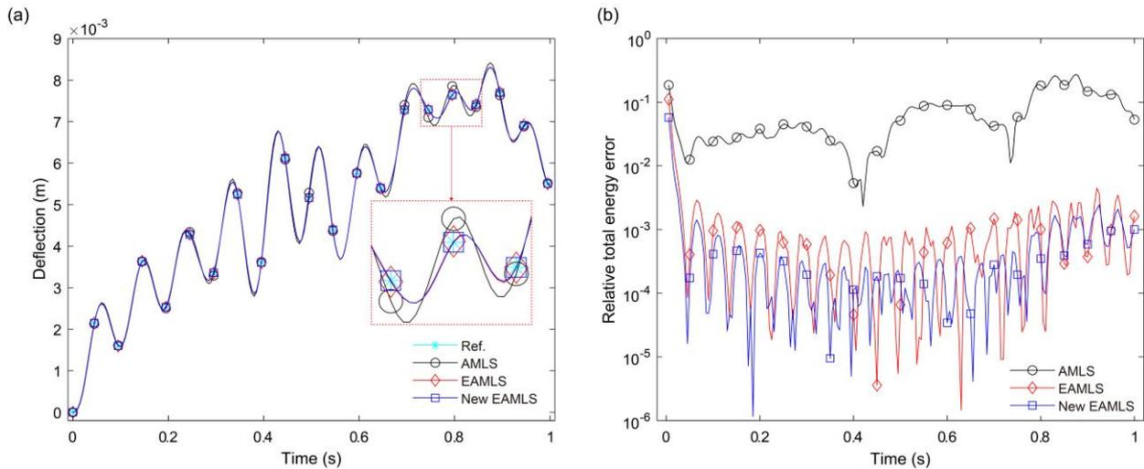
Fig. 4. Transient response for the cantilever plate: (a) deflection at the free end and (b) relative total energy errors.
