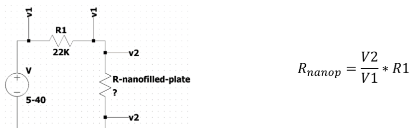
Fig. 11 experimental set-up circuit scheme and sensor resistance equation
