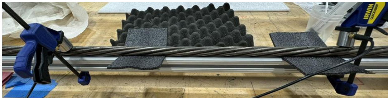
Fig. 4 Reference ultrasound NDE experiment along Strand 0
