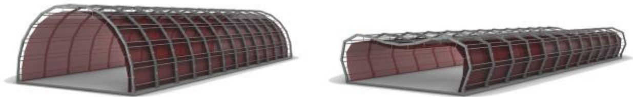
Fig. 1 Reconfigurable building structure of a rigid bar linkage system presented in (Phocas 2020)
