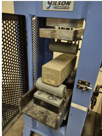
Fig. 5 Beam test setup
