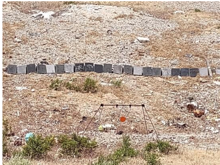
Fig. 3 UHPC panels placed in the field prior to testing
