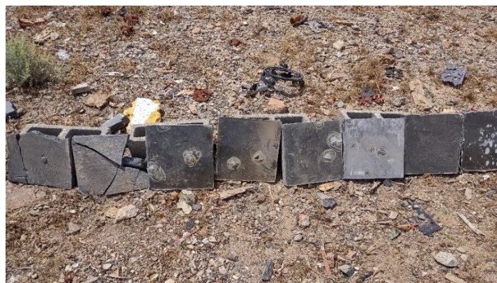
Fig. 4 UHPC panels after testing
